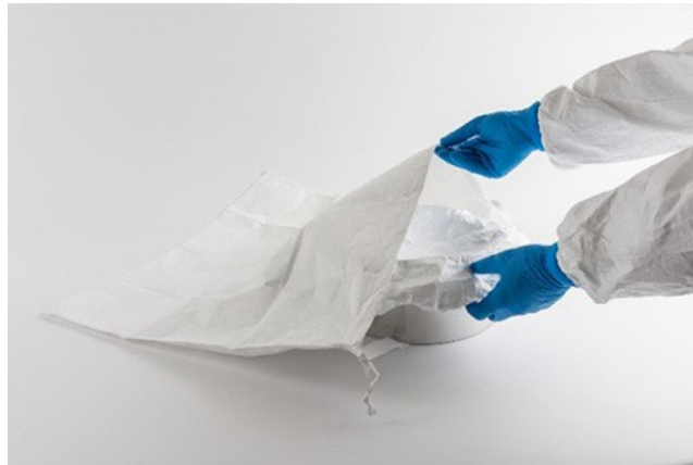
Figure 2: A stopper bowl is placed into a sterilization bag
